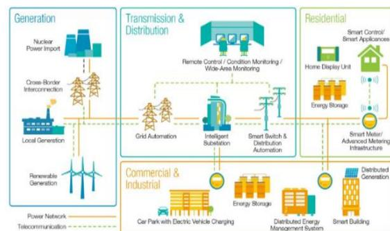
**Figure 1:** How SG connects between Generations, Transmission and Residential
